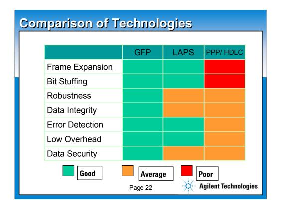
This slides provides a comparison of GFP, LAPS and PPP/HDLC.
