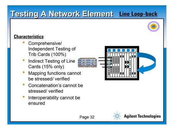
Today the commonly used testing technique is by looping back the Line Side. This capability provides you limited visibility of the device being tested.
