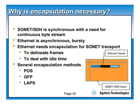
So why is it necessary to encapsulate Ethernet to transport it over SONET/SDH?
