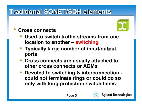
The second basic SONET/SDH device is a cross-connect, which is used to switch a traffic stream from one location to another so that a circuit or part of a circuit is completed. Cross-connects usually have a large number of ports and will be connected to ADMs in a ring topology or perhaps to another cross-connect on another ring.
