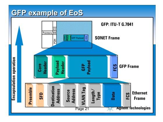
In principle the operation of the encapsulation technologies are very similar. In this example we look at how an Ethernet frame ends up in a Generic Framing Procedure encapsulation
