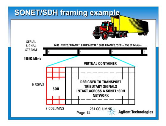
SONET/SDH works on a hierarchical framing system where a mix of different transmission channels can be placed in logical transmission containers and transported across a network section.
