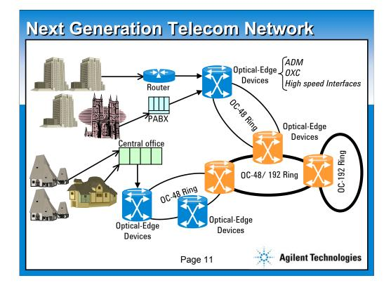
This diagram outlines typical application of Next Generation SONET Device. As you can see a Next Generation SONET Devices combines the traditional SONET/SDH functions of ADMs and OCXs in a single device.it also integrates the data functions with telecom networks. High speed interfaces like GbE are also supported on these devices. The basic design architecture of these devices provides them to serve both data and voice with same efficiency.
