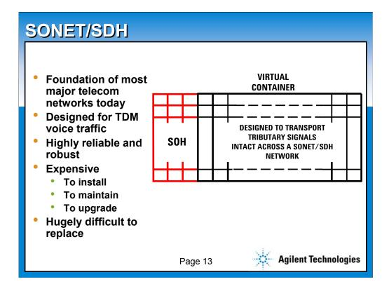
Our first port of call is the SONET or SDH systems of hierarchical TDM transmission.
