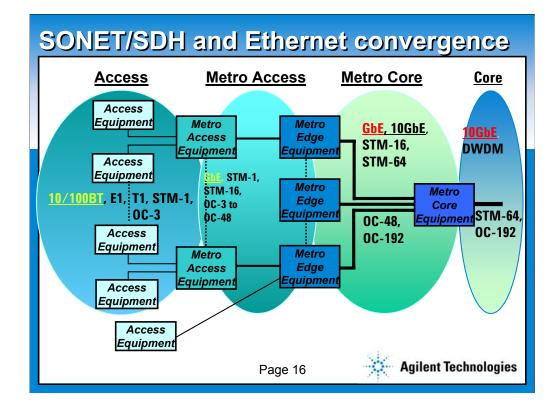
The second of the enabling technologies is Ethernet. Ethernet is now present in every segment of the network, particularly the metro networks. This means that network elements at every point in the network must support Ethernet and the SONET/SDH technologies.
